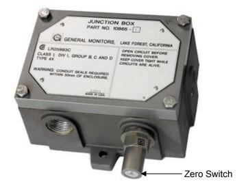
**Zero the Unit**. To insure a true zero and maintain IR700 accuracy, the IR700 must be purged with nitrogen for a sufficient time to remove all naturally occurring carbon dioxide. Apply the General Monitors magnet that was included with the unit to the Zero Switch / LED for approximately three seconds. The LED in the switch will light to show proper placement.
