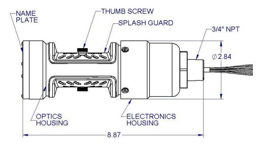
Figure 10: Outline and Dimensional Drawing, IR700, inch measurements
