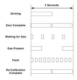
Figure 8. IR700 Zero Switch / LED During Zeroing and Calibration
